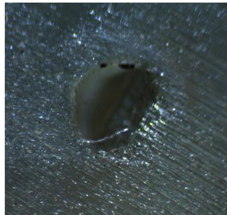
**Figure 6.** Single hole with 0.8 mm diameter.
