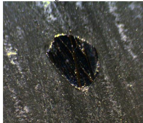
**Figure 10.** The appearance of a single hole with a defect in shape at the sample boundary (in the volume the hole has a cylindrical shape) after filling with Wood alloy. Hole diameter is 1.2 mm.
